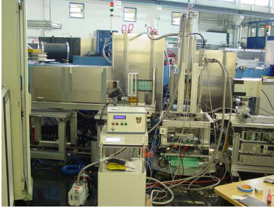
Figure 1: The MIEZE setup at MIRA. The \pi -flipper coils are contained within the \mu -metal box on the left hand side, followed by the polarisation analyser (blue box) and the sample inside a magnet. On the right the detector on its x,y,z-support is shown.
