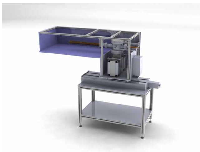
Figure 2: Schematic overview of our all-metal sealed horizontal RF heated cold-boat system including baking tent.
