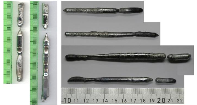
Figure 2: Overview over the \text{Nb}_{1-y}\text{Fe}_{2+y} single crystals grown by the vertical-zone-melting technique. Vertical on the left are the 2 crystals grown in the first period with nominally stoichiometric composition. Horizontally aligned on the right are the 4 crystals with varying composition grown in the second period.
