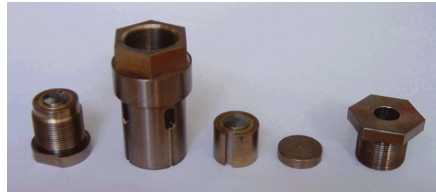
Figure 1: Parts of the Bridgman cell: the bottom screw with the lower anvil (a) is fixed tightly to the cell body (b). The electrical leads leave the pressure cell through the windows in the cell body. The piston with the upper anvil (c) is pushed up-side down the cylinder towards the lower anvil by an external force generating mechanism via the hole in the top screw. The plate (d) is placed between the piston and the top screw to reduce stress during tightening the top screw (e).
