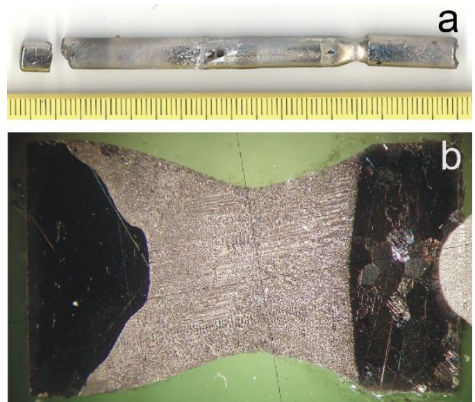
Figure 2: a) As grown Mn 3 Si crystal. b) Longitudinal cut through final zone of the Mn 3 Si crystal.
