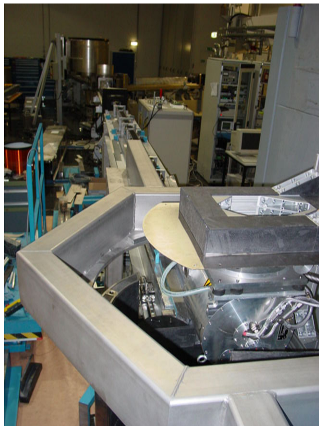
Figure 1: The velocity selector and the neutron guide leading towards RESEDA.
