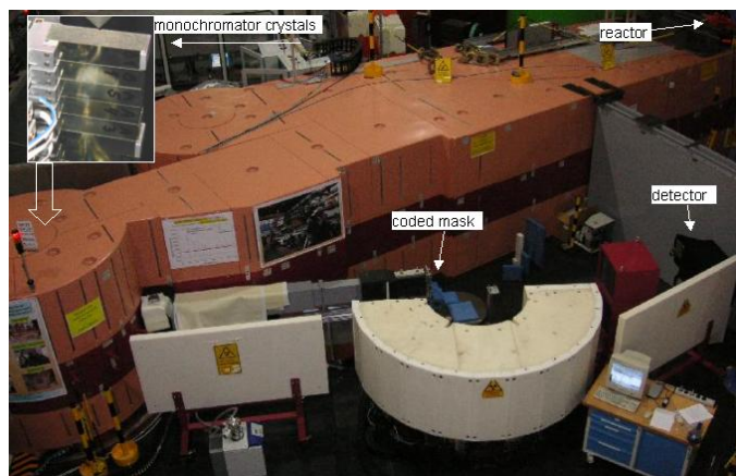
Figure 2: Setup at the powder diffractometer SPODI
