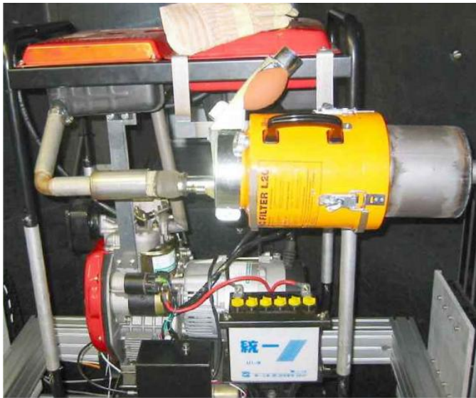
Figure 1: Diesel combustion engine for the neutron radioscopy at FRM-II
