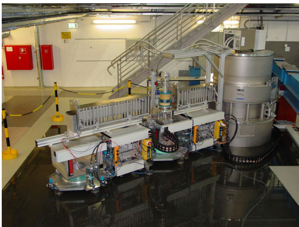
Figure 1: MIRA in the polarised reflectometer option equipped with a magnet and a closed cycle cooling machine.
