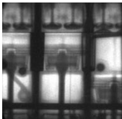
Fig. 1: Two images of the running cycle of a motorbike at 800 rpm, 250ms with 60 image accumulations
