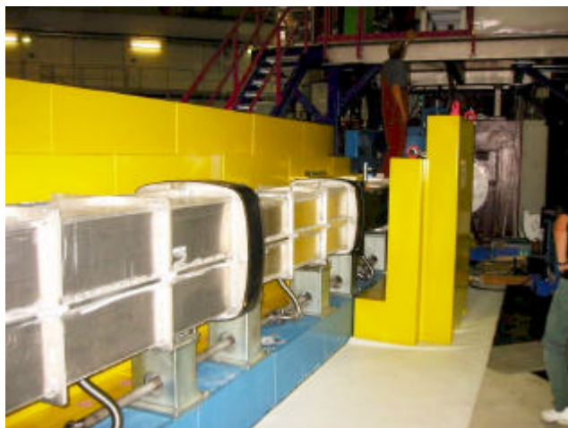
Fig. 6: The flight tube with convex flanges
