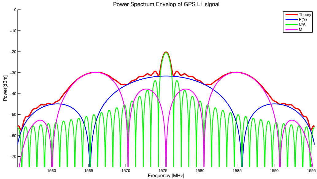
Figure 2.6: Generated envelope of power spectrum of GPS L1 for BIIRM satellites (uncalibrated)
