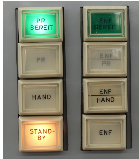
Figure 2.2: Mode selection panel of the Reglergestell . The ENF button is a German abbreviation for Eigennachführung and selects the auto-tracking functionality.
