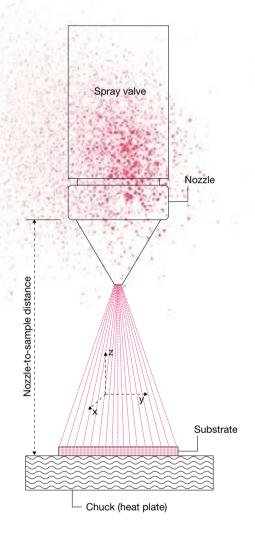
The basic principle of the high-tech spray nozzle is not unlike conventional air brushing. But here, everything must be perfect to ensure that extremely thin layers can be applied evenly. The Munich-based researchers have become adept at producing homogeneous inks from the exotic substances, adhering them to the substrate and achieving a perfectly even spray film.
