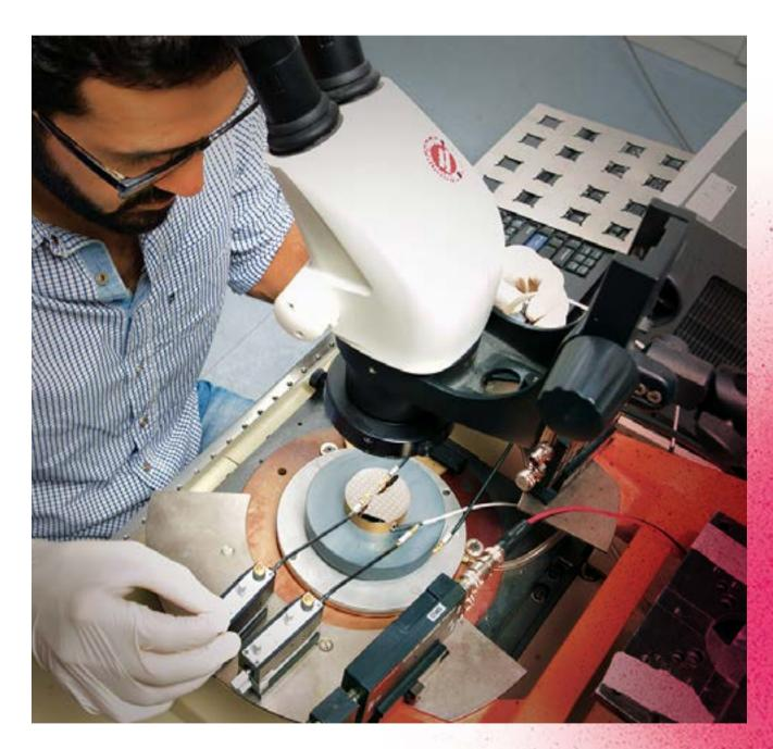
Patience and care are needed when developing the delicate structures. The TUM researchers use inkjet printing to manufacture the electronic circuits for the sensors. Here, Dr. Alaa Abdellah uses a microscope to connect one of the tiny transistors to a carbon-nanotube-coated sensor in order to test its electrical properties.
