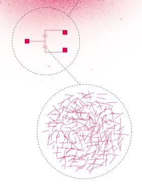
When viewed under the microscope we can see that the structures of the sensors (center) are composed of extremely fine carbon nanotubes (bottom) that form a dense mesh when deposited onto a surface. With their spray method, the TUM researchers can layer them onto films in large quantities (top).
