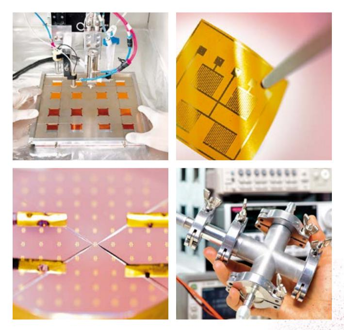
**Tried and tested:** Coatings are applied to a film in the spray chamber (top left). The template ensures that the correct shape is maintained. The finished part – in this example, a prototype for a flexible gas sensor based on carbon nanotubes (top right) – will first be tested for its electrical properties (bottom left), followed by further testing for its sensing functionality with a variety of gases (bottom right).
