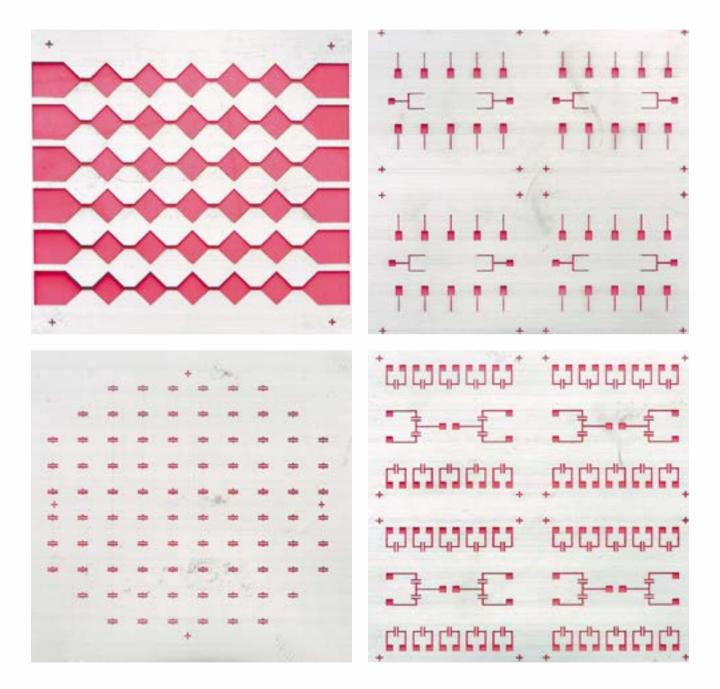
It all begins with simple shapes stamped onto templates. The researchers use these to see whether the exotic materials that they spray onto films will adhere properly and distribute evenly without running off. Later, when they are working on industrial applications, they must ensure that the spray coating has been applied precisely. This is the only way to ensure that the delicate sensor structures function correctly.
