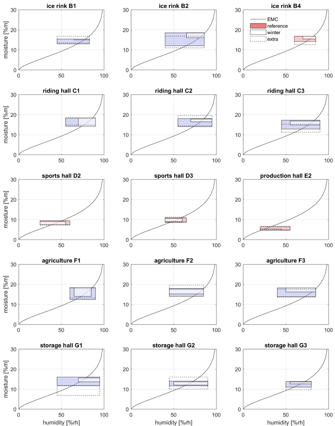
Figure 6: Comparison of year-through operation and summer operation of different heated (red) and non-heated buildings (blue)
