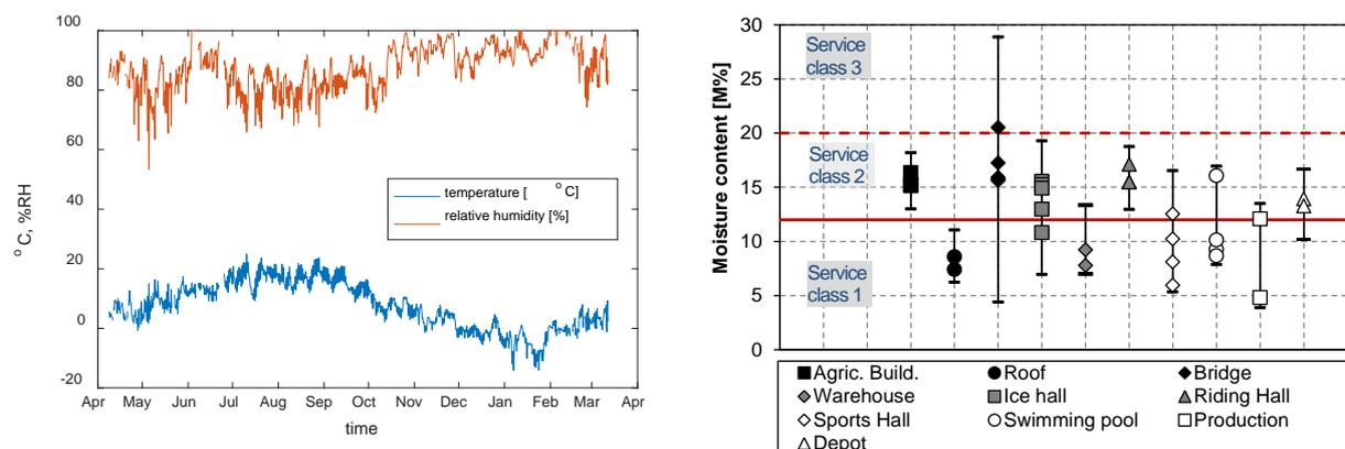
Figure 1: Measured yearly ambient climate around the Obermatt Bridge located near Langau im Emmental (CH) (left) and the plotted of average moisture content obtained from different building types and structures (right) [7][9] with relation to the Service Classes (SC) according to Eurocode 5 [8].
