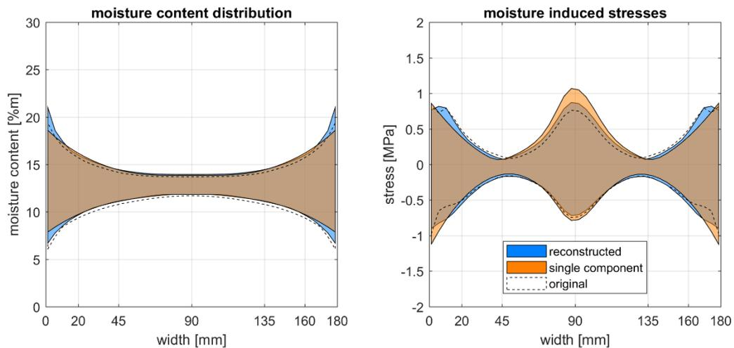
Figure 11: Comparison of envelopes of moisture content distribution and moisture induced stresses using the reconstructed climate, a single frequency component, and the original climate.
