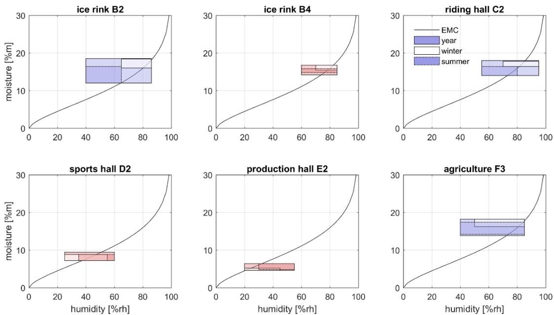
Figure 7: Comparison between the total year-through envelope, the winter and summer envelopes of measured humidity and moisture content in different buildings.
