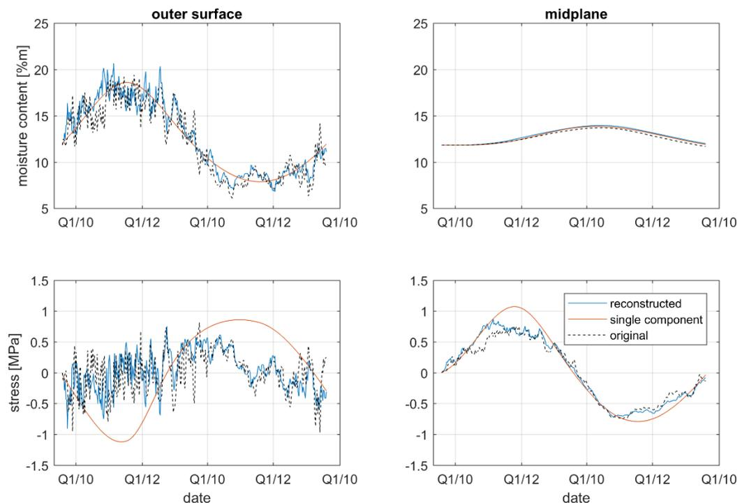
Figure 12: Comparison of moisture content distributions and moisture induced stresses using the rebuilt climate and the original climate on a cross section of 180 mm wide
