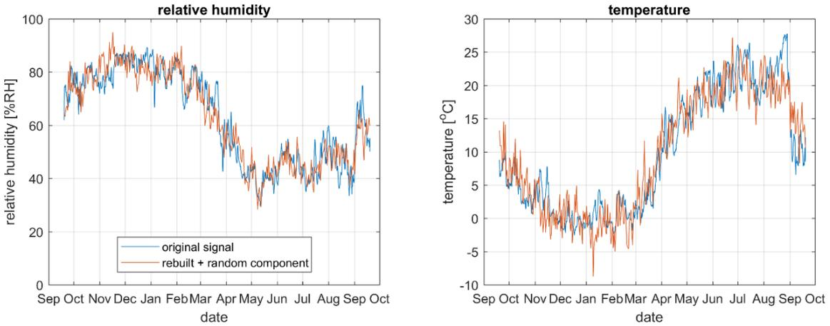
Figure 10 : Reconstructed relative humidity (left) and temperature (right) using the eight frequency components, amplitudes, and phases, along with the average and random distribution of daily effects.
