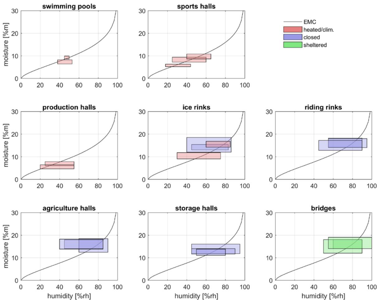
Figure 4: Comparison of measured relative humidity with the measured moisture content at 15 mm depth, moisture in the bridges shows a range of reasonable moisture contents that are to be expected at different depths.
