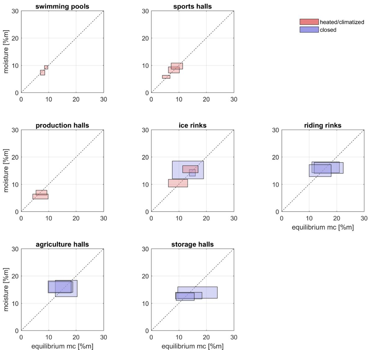
Figure 5: Comparison of minimum and maximum EMCs at the surface with the moisture contents measured at 15 mm depth of the monitored buildings.
