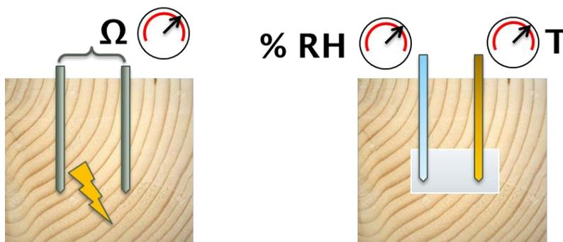
Figure 8: Illustration of moisture content measurement using the resistance method (left) and the measurement of climate within a small void (right)
