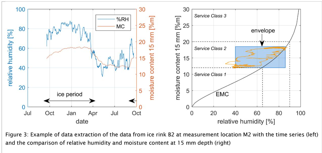
Figure 3: Example of data extraction of the data from ice rink B2 at measurement location M2 with the time series (left) and the comparison of relative humidity and moisture content at 15 mm depth (right)
