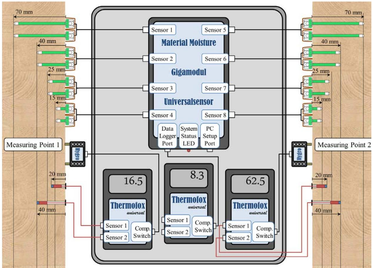
Figure 2: Example setup used for the measurement of moisture content, including pin type gauges for the measurement of moisture content (green), climate (hygro sensors) and temperature sensors (red), and logging equipment [9].
