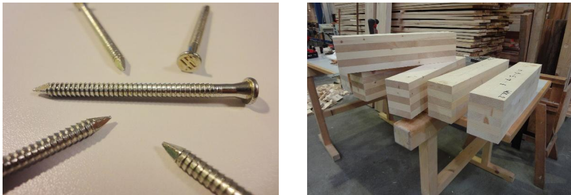
Figure 2. Simpson Strong-Tie annular ringed shank nail (left) and CLT specimens used for withdrawal tests (right).
