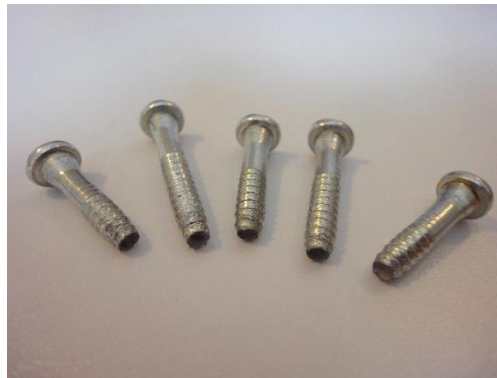
Figure 7. Failure modes of the uniaxial tension tests.
