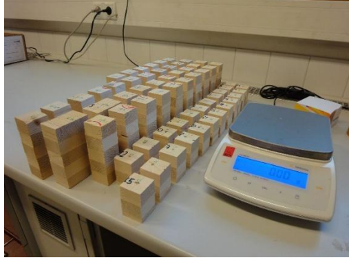
Figure 6. Samples used to determine moisture content and density of the CLT panels.
