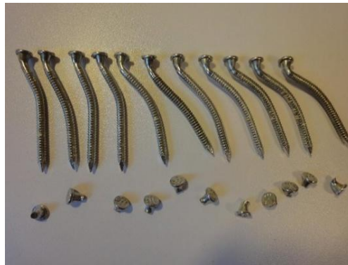
Figure 12. Deformed fasteners after shear tests.
