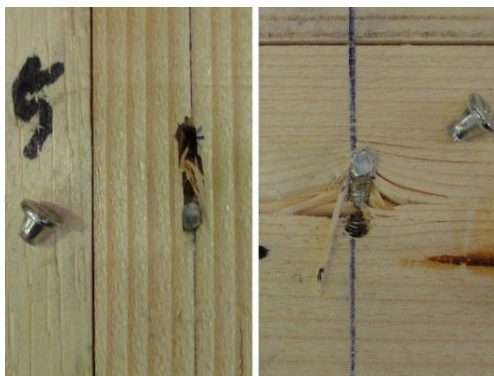
Figure 13. Damaged embedment after shear tests.
