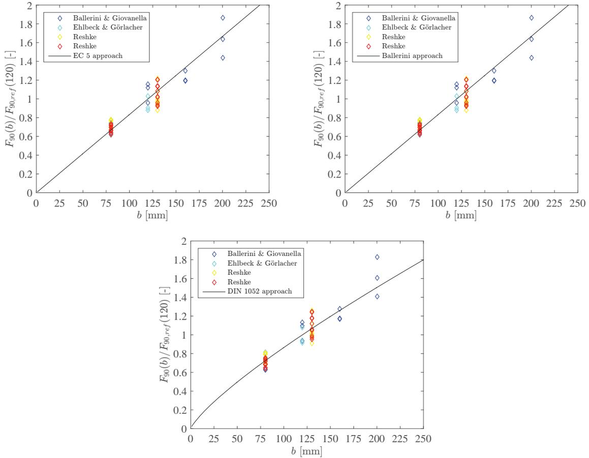
**Fig. 15:** Impact of beam width  $b$  on the relative load-carrying capacity with a reference to  $b = 120$  mm.
