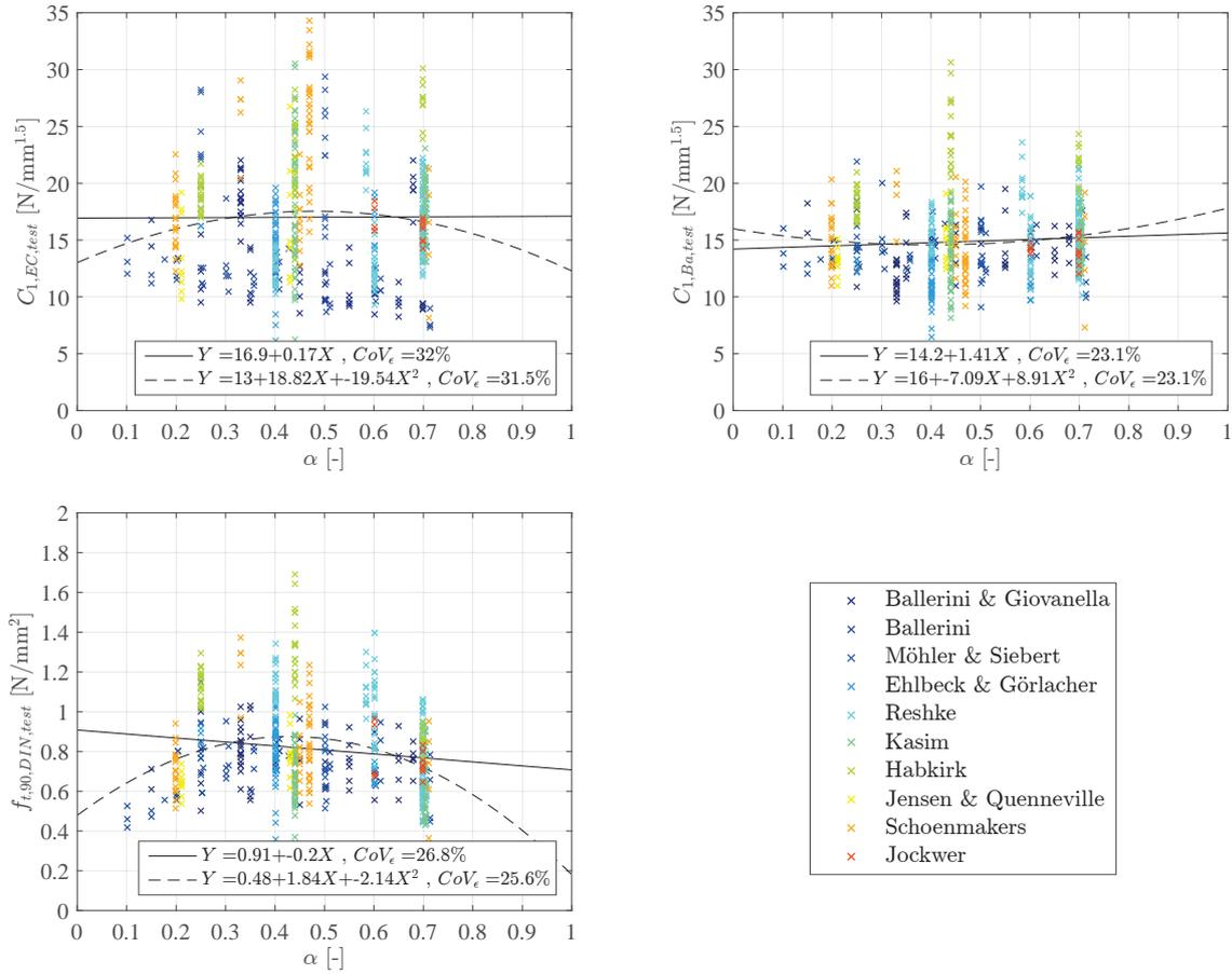
**Fig. 22:** Evaluation of the material strength parameters according to test results with regard to the relative connection height  $\alpha$ .
