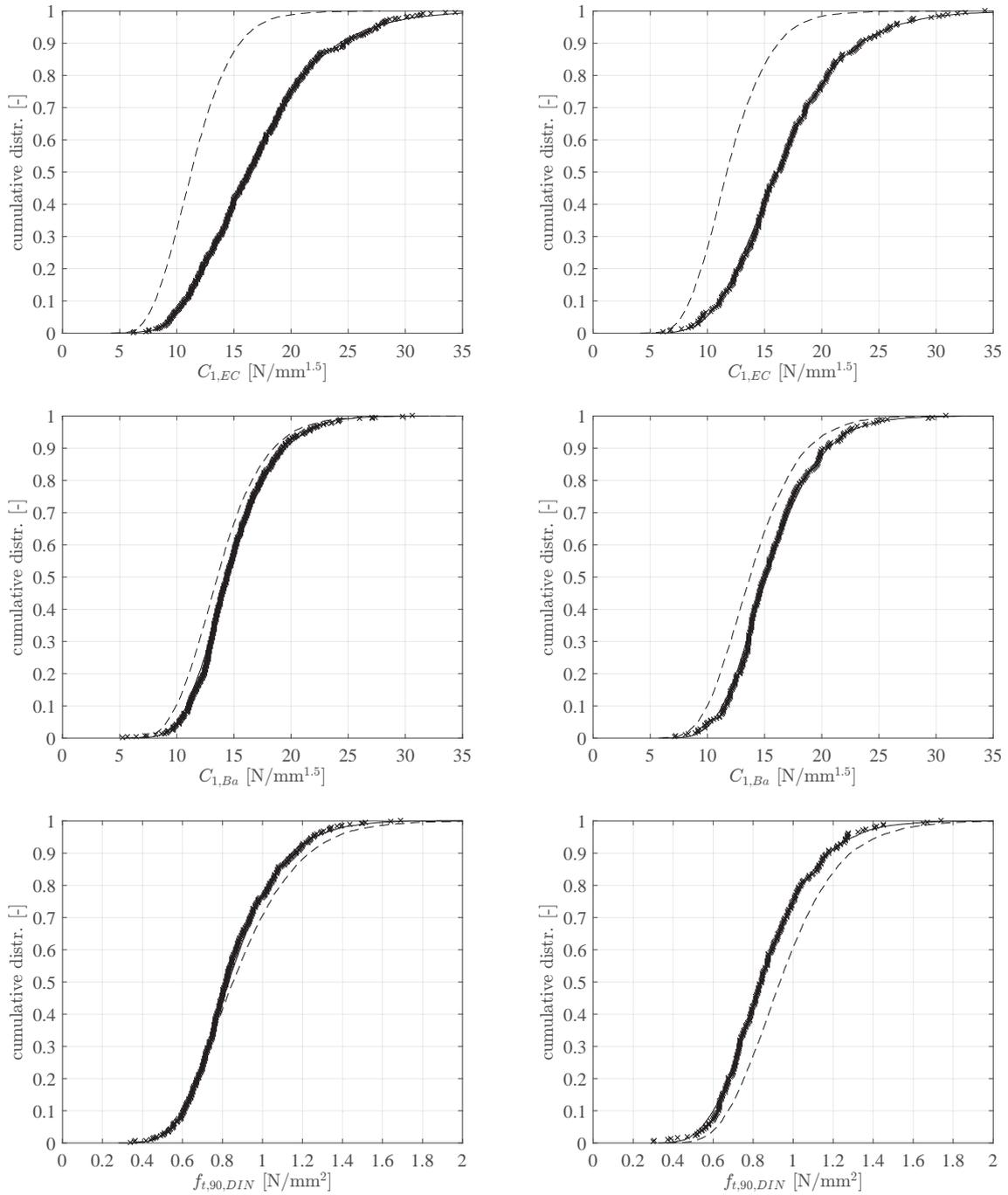
**Fig. 25:** Cumulative distribution of the material parameters  $C_{1,EC}$ ,  $C_{1,Ba}$  and  $f_{t,90,DIN}$  and lognormal distribution function for the best or second best fit for glulam (left) and solid timber (right).
