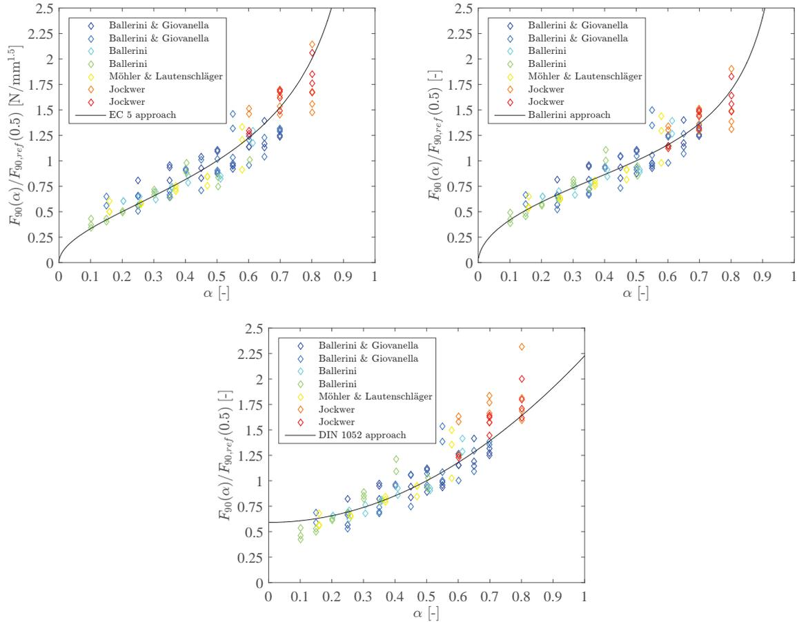
**Fig. 16:** Impact of relative connection height  $\alpha$  on the relative load-carrying capacity with a reference to  $\alpha = 0.5$ .
