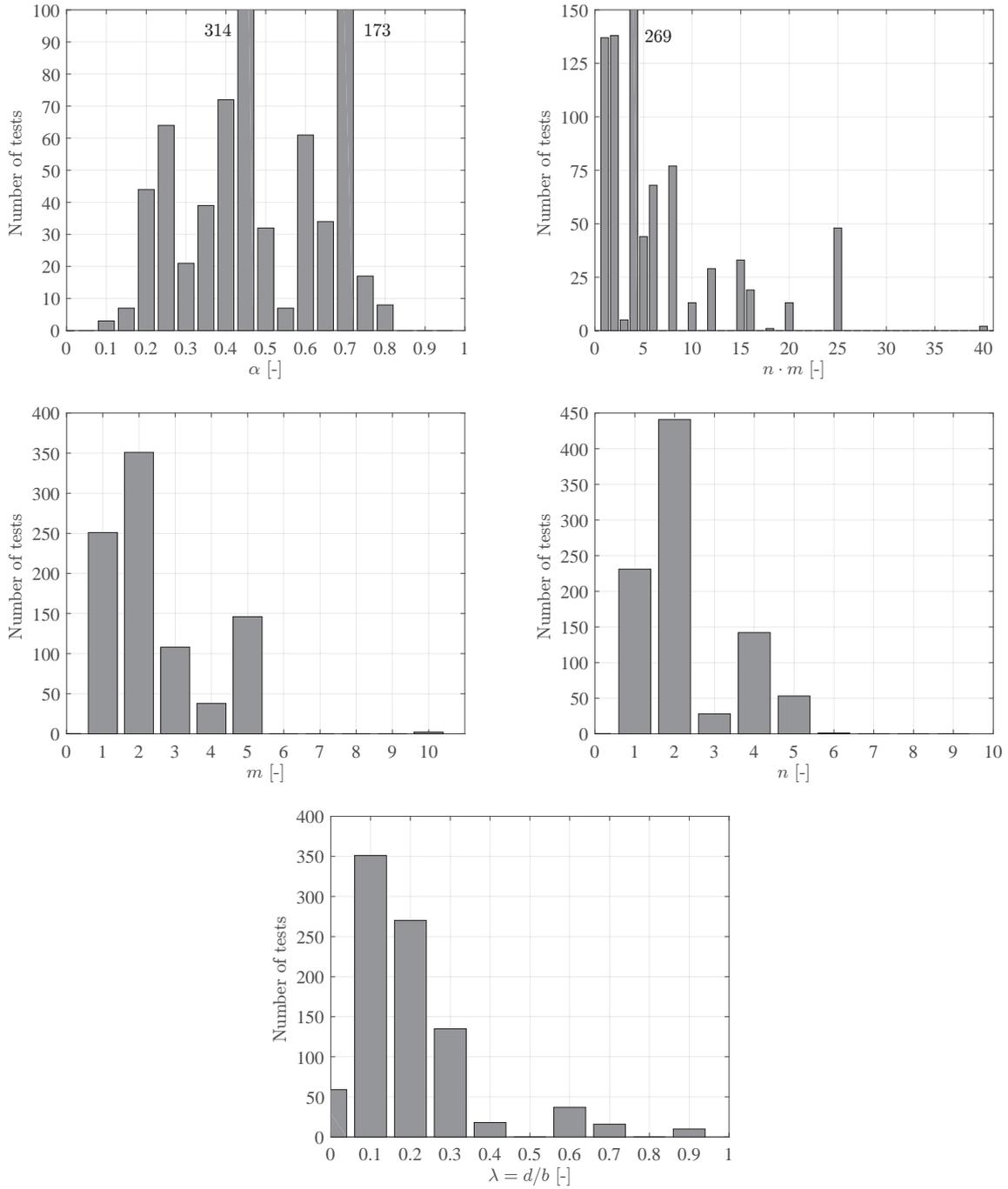
**Fig. 13:** Histograms of beam and connection parameters relative connection height  $\alpha$ , number of fasteners  $m \cdot n$ , number of fastener columns  $m$ , number of fastener rows  $n$  and slenderness of the fasteners  $\lambda = d/b$  as studied in the publications listed in Tab. 3.
