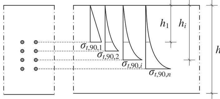
**Fig. 3:** Distribution of tension perpendicular to grain stresses in different rows  $n$  of the connection according to Möhler and Siebert (1980)
