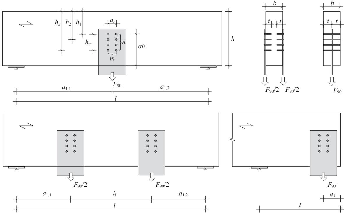
**Fig. 1:** Definition at connections loaded perpendicular to grain.
