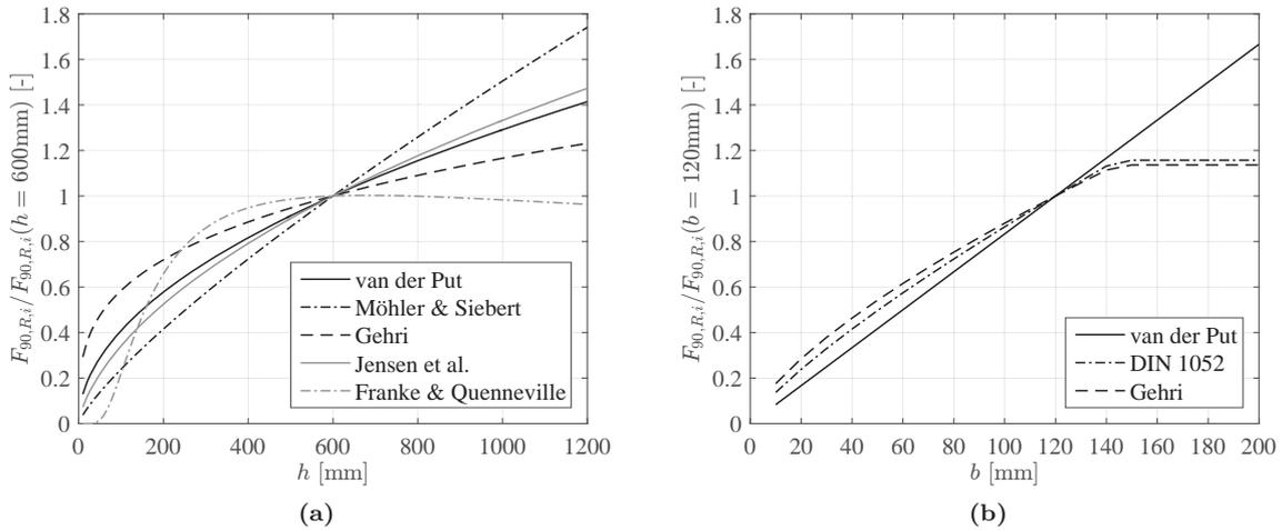
**Fig. 9:** Impact of the beam height  $h$  (a) and beam width  $b$  (b) on the relative load-carrying capacity in the approaches.
