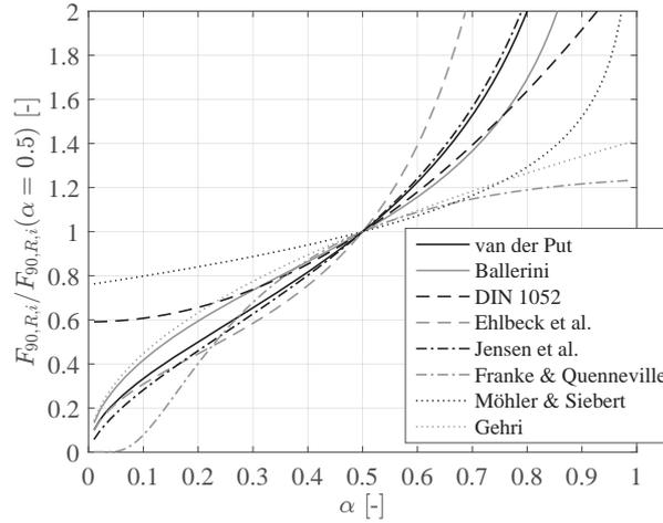
**Fig. 10:** Impact of the relative connection height  $\alpha$  on the relative load-carrying capacity.
