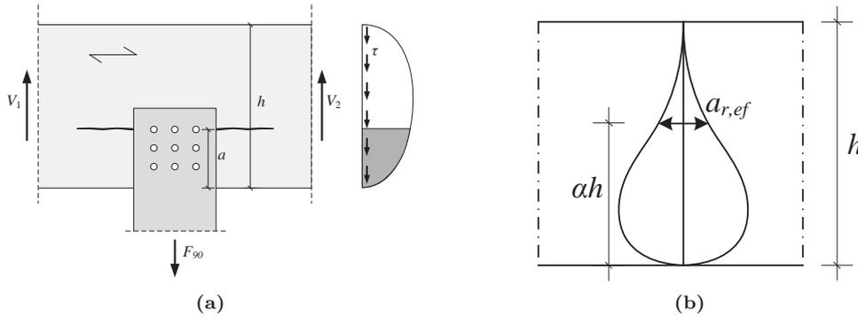
**Fig. 4:** Impact of the relative connection height  $\alpha$  on tension perpendicular to grain stresses (a) and impact of the width of the connection (b) according to Ehlbeck et al. (1989)
