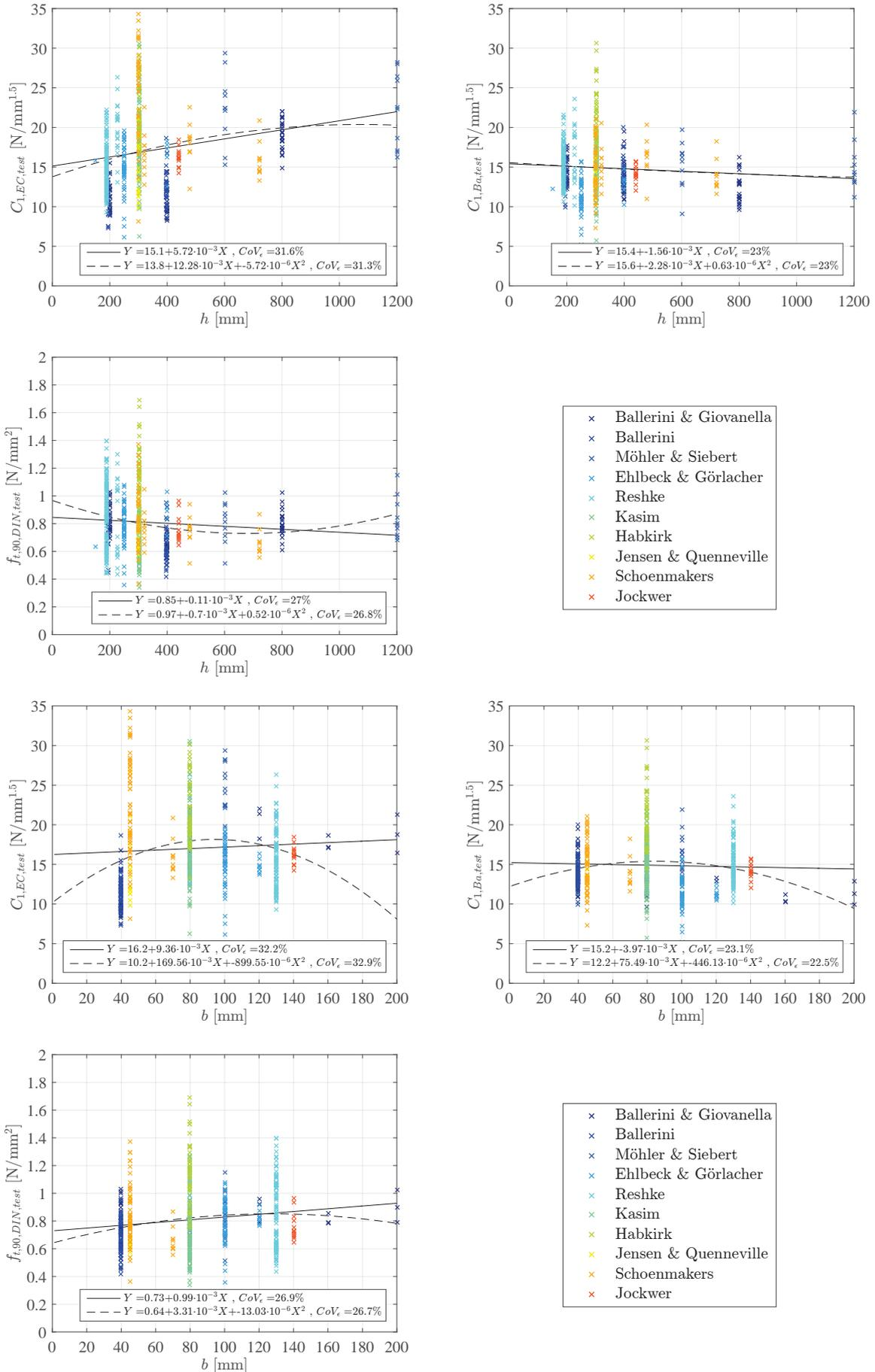
**Fig. 21:** Evaluation of the material strength parameters according to test results with regard to the beam height  $h$  and the beam width  $b$ .
