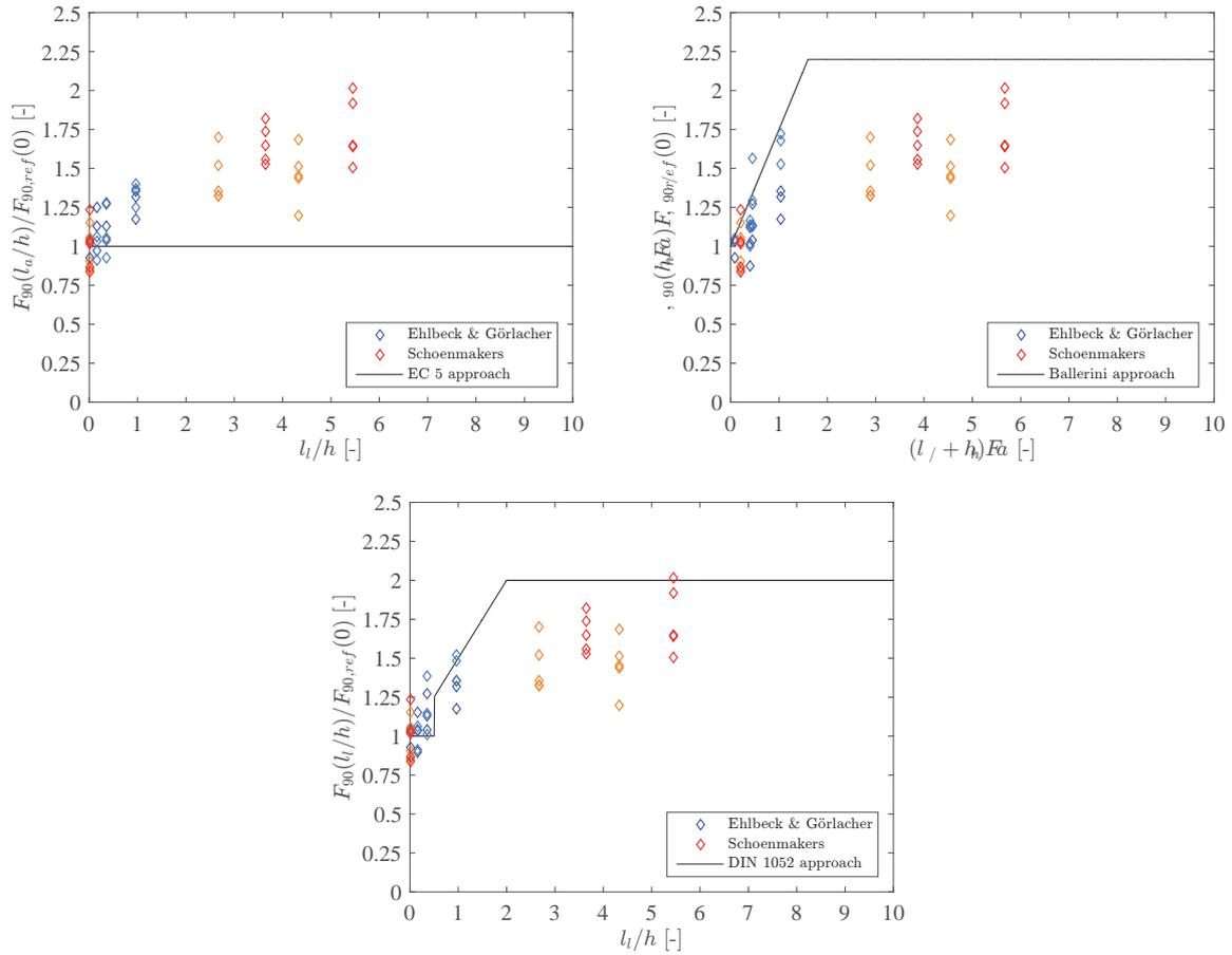
**Fig. 20:** Impact of the distance between connections  $l_l$  on the relative load-carrying capacity.
