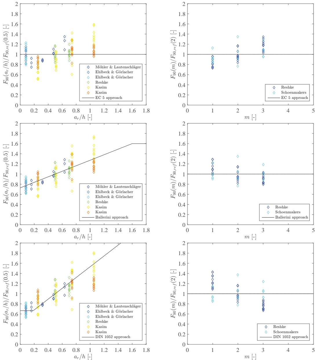
**Fig. 17:** Impact of connection width  $a_r/h$  and number of fastener columns  $m$  on the relative load-carrying capacity with a reference to  $a_r/h = 0.5$  and  $m = 2$ .
