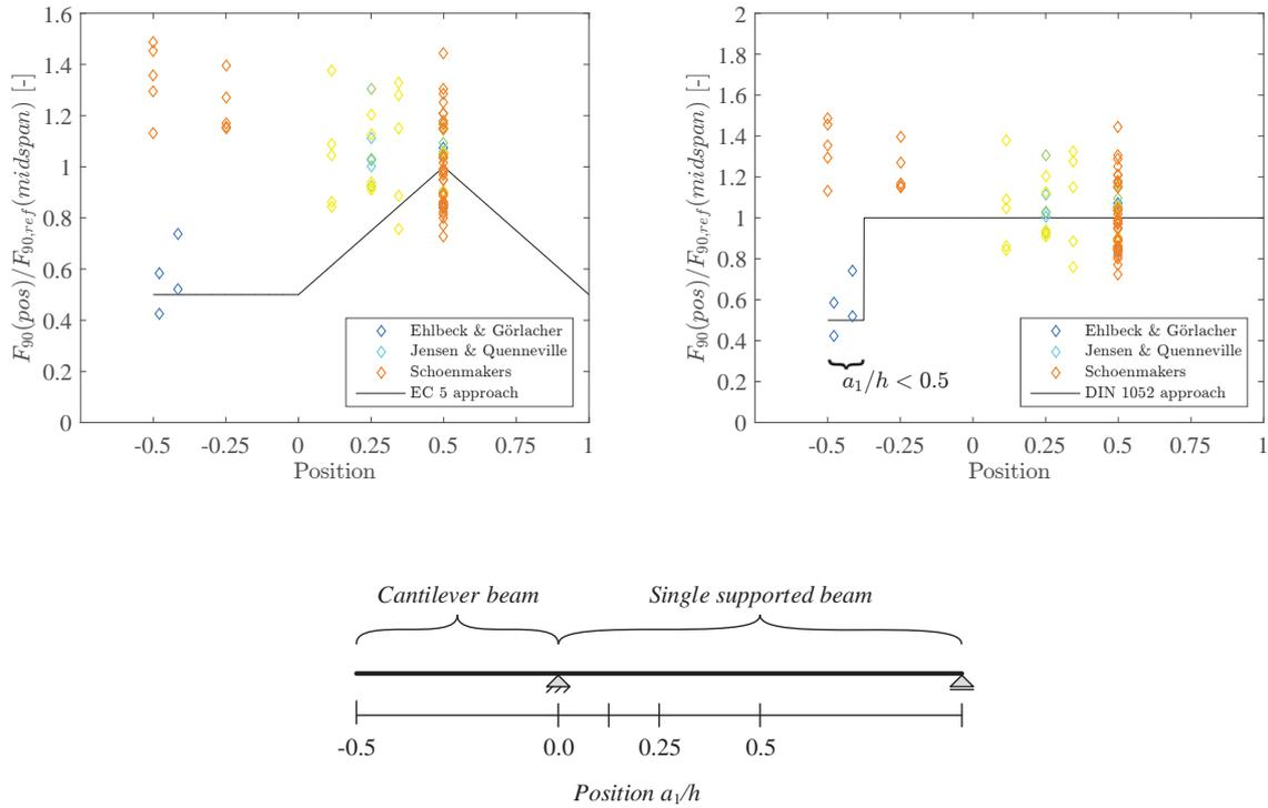
**Fig. 19:** Impact of the position  $a_1/h$  of a connection on the relative load-carrying capacity with a reference to  $a_1/h = 0.5$  for single supported beams.
