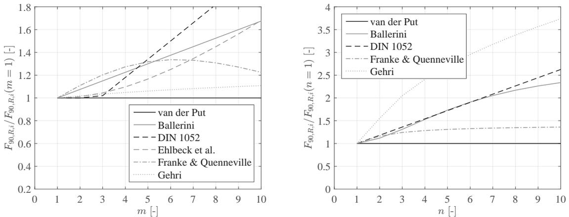
**Fig. 11:** Impact of the width of the connection  $a_r = 5d(m - 1)$  with the number of fastener columns  $m$  (left) and the height of the connection  $h_m = 3d(n - 1)$  with the number of fastener rows  $n$  (right) on the relative load-carrying capacities  $F_{90,R,i}/F_{90,R,i}(ref)$ .
