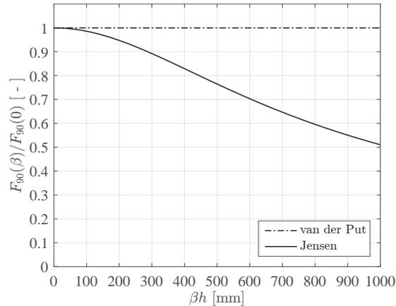
**Fig. 7:** Relative reduction of crack propagation load with increasing crack length  $\beta h$  for  $\alpha = 0.6$ ,  $E = 11500 \text{ N/mm}^2$  and  $G = 650 \text{ N/mm}^2$ .
