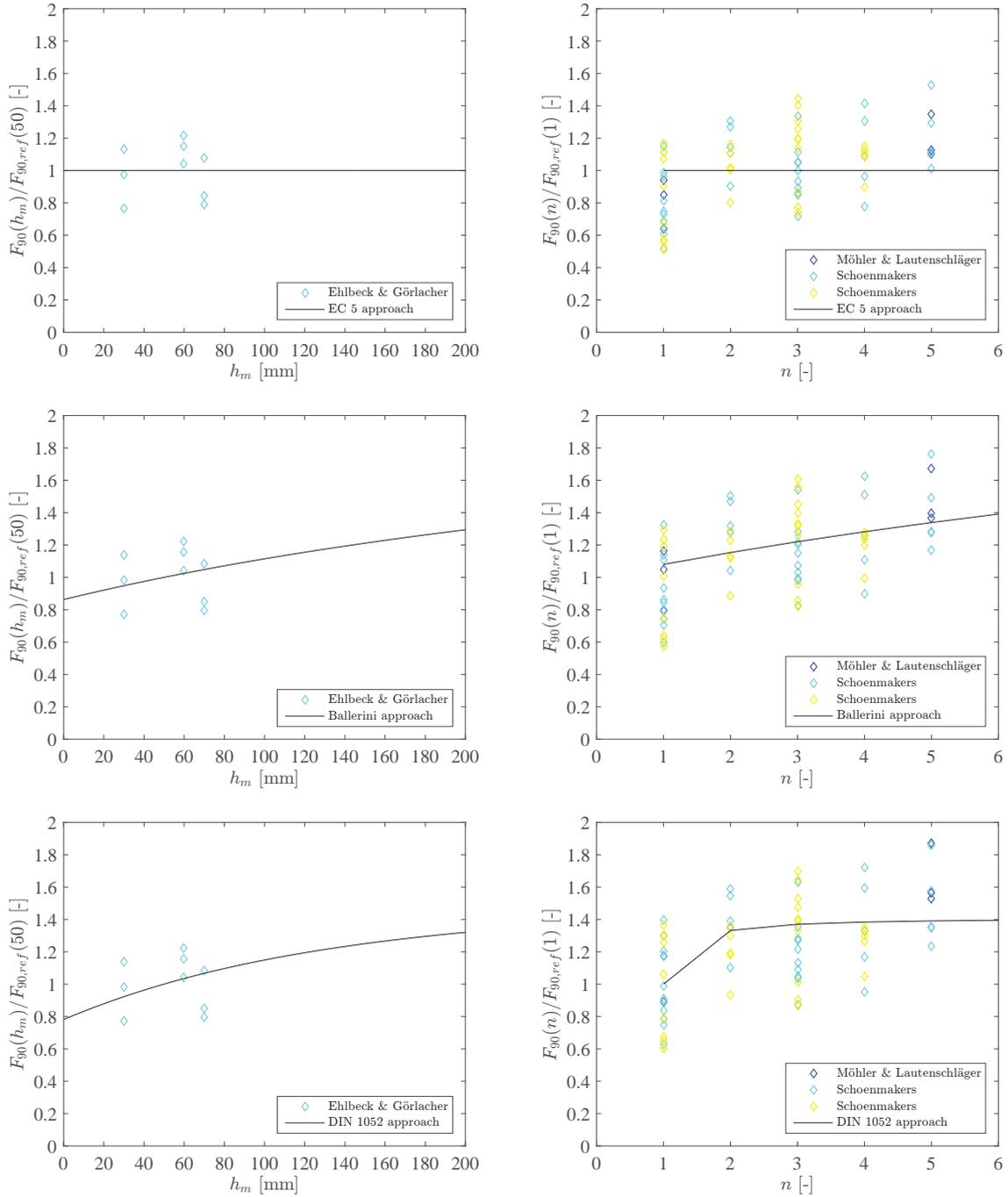
**Fig. 18:** Impact of connection height  $h_m$  and number of fastener rows  $n$  on the relative load-carrying capacity with a reference to  $h_m = 50$  mm and  $n = 1$ .
