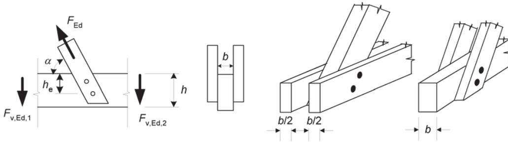
**Fig. 8:** Connection loaded at an angle to the grain according to EC5 (CEN 2004).
