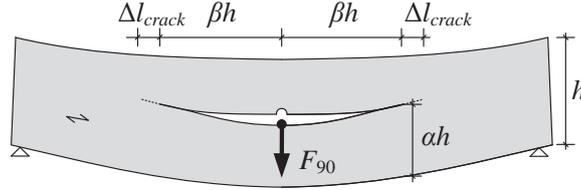
**Fig. 6:** Model of a beam with a connection perpendicular to the grain and a crack propagating at a single fasteners.
