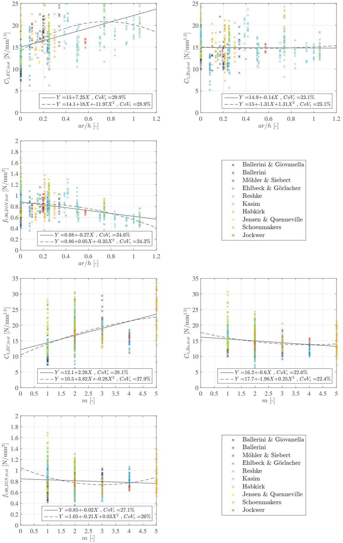
**Fig. 23:** Evaluation of the material strength parameters according to test results with regard to the relative connection width  $a_r/h$  and the number of fastener columns  $m$ .
