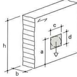
**Fig. 5:** Effective width  $b_e$  in dependency of the diameter and type of the fastener and denotations of the geometrical parameters at a connection loaded perpendicular to the grain according to (Lignum 1990).
