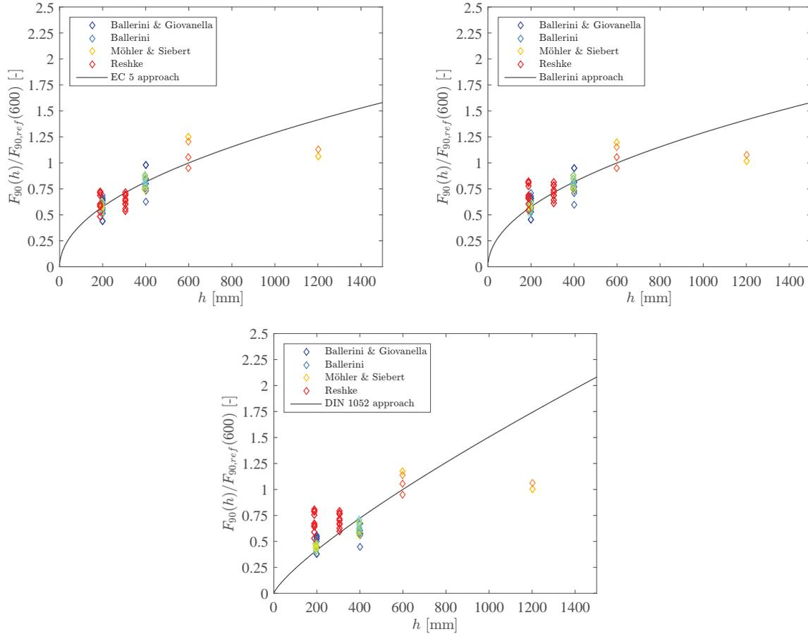
**Fig. 14:** Impact of beam height  $h$  on the relative load-carrying capacity with a reference to  $h = 600$  mm.
