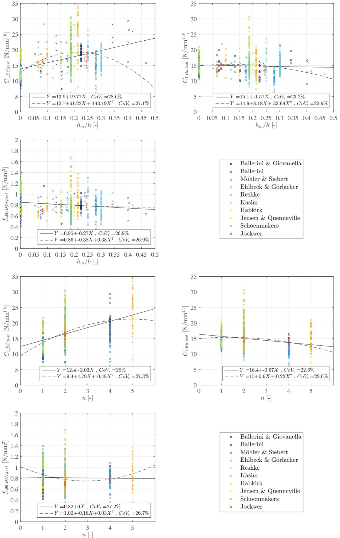
**Fig. 24:** Evaluation of the material strength parameters according to test results with regard to the connection height  $h_m/h$  and the number of fastener rows  $n$ .
