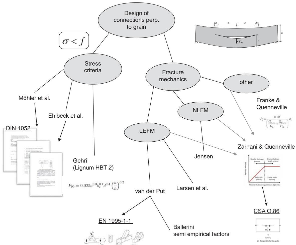
**Fig. 2:** Illustration of the background of design approaches for connections loaded in tension perpendicular to the grain.
