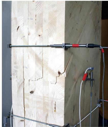
*Fig. 11 Gross-shear failure in specimen D2-3 (fatigue loading)*
