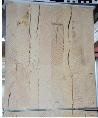
*Fig. 9 Cracks in x – y-plane in specimen D2-1 (fatigue loading)*
