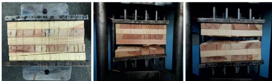
*Fig. 9 Typical failures of CLT specimens*
