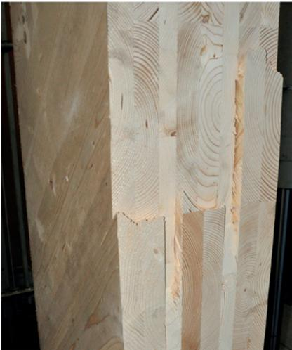
*Fig. 10 Gross-shear failure in specimen S1-2 (static loading)*
