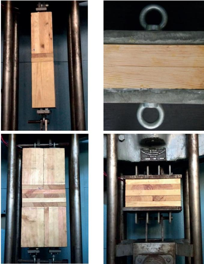
*Fig. 6 Test arrangements for small specimens (top) and CLT specimens (bottom)*
