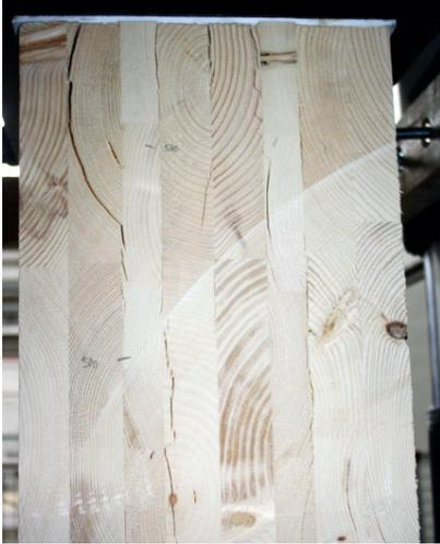
*Fig. 8 Cracks in x – y-plane in specimen D1-3 (fatigue loading)*
