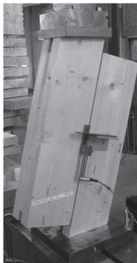
Fig. 6. Test set-up as proposed by Hirschmann for net shear tests of single nodes
