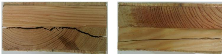
b) perpendicular glued boards (type B)
