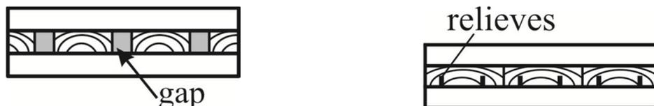
Figure 8: Gaps and relives in CLT cross section
