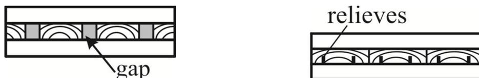
Figure 8: Gaps and relieves in CLT cross section
