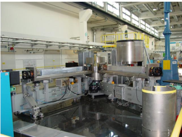
Figure 1: The image shows the two secondary spectrometer arms of RESEDA. The open mumetal shielding gives free view on the NSE and NRSE coils.
