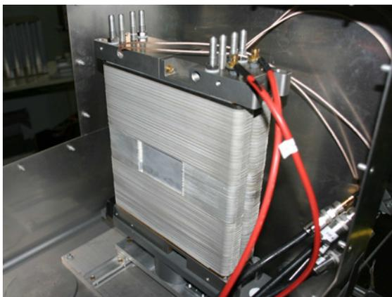
Figure 2: One of MIRA's NRSE bootstrap coils, mounted inside the magnetic shielding and on top of the positioning mechanics.
