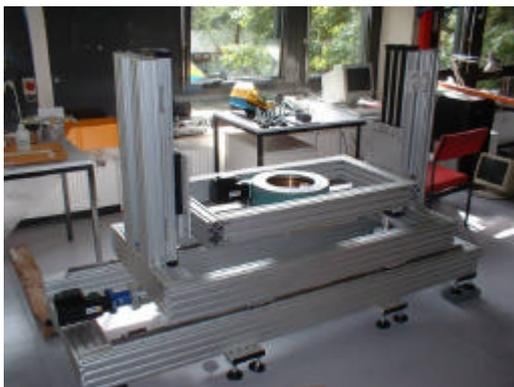
*Fig. 10: The sample manipulator*
