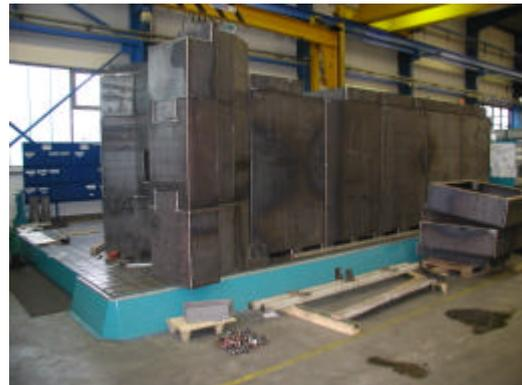
*Fig. 12: Part of the flight tube shielding and entrance to the measurement cabin*
