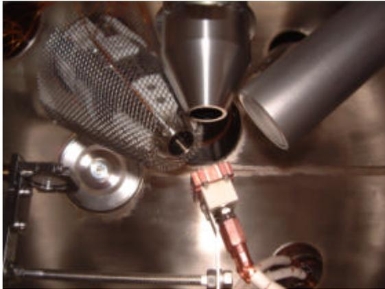
Fig. 2: View into the analysis chamber. The incoming positrons are focused by electric lenses (top left) onto the sample in the center of the analysis chamber. Top: entrance of the electron energy analyzer. Top right: tungsten shielded NaI-detector.
