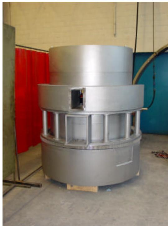
Fig. 1: The shielding for the monochromator of MIRA
