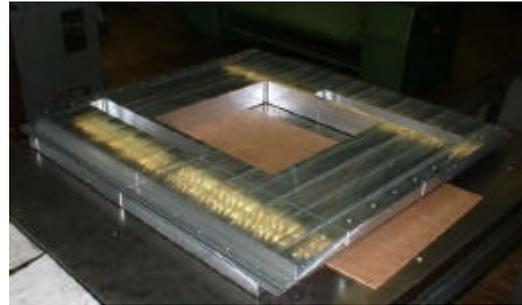
*Fig. 11: The frame of the beam size limiter*
