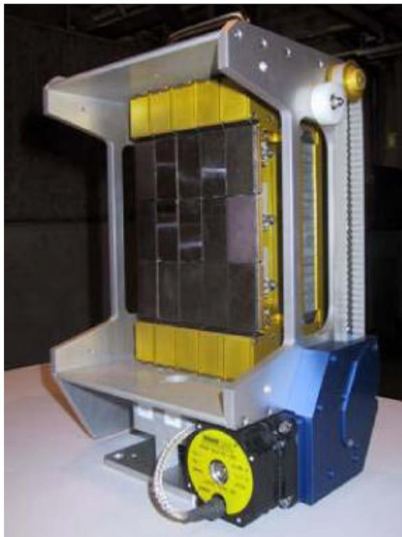
*Fig. 2: Picture of the new Heusler analyzer assembly. As explained in the text the 3 columns of the analyzer are magnetized individually to allow horizontal focusing.*
