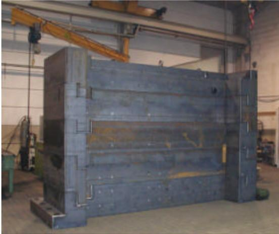
*Fig. 14: A side wall of the measurement cabin made from stacked segments*
