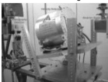
Fig. 1: Positioning of the velocity selector at the PGA beam line for neutron radiography and tomography purposes.
