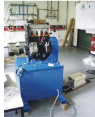
Fig. 2: Test stand for the combustion engine
