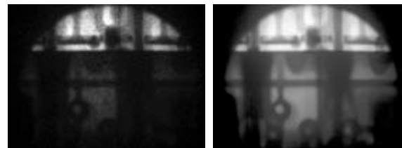
Fig. 3: A single frame (left) contains only 14 graylevels and a summed NR-image after processing (right).
