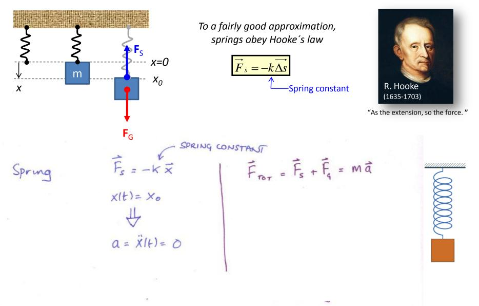
This alternative "mode" of motion can be easily studied by looking at a mass attached to a spring on a frictionless surface (e.g. air hockey table)
