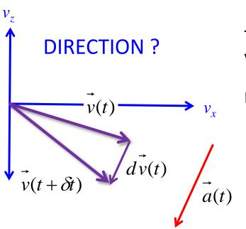
The instantaneous acceleration (*Beschleunigung*) is a vector orientated parallel to  $d\mathbf{v}(t)$
