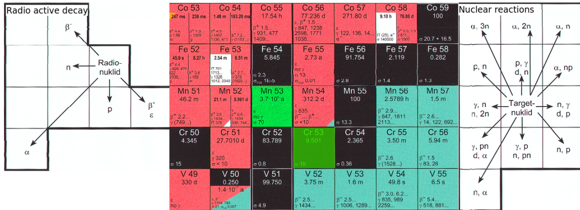
Figure 5.6: Chart of nuclides with radioactive decay and nuclear reactions scheme. ^{53}\text{Mn} and its isobar ^{53}\text{Cr} are highlighted.
