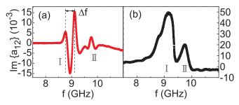
FIG. 4. (a) Imaginary part of the transmission signal obtained on CoFeB when the applied field of  $1.9\,\mathrm{T}$  is perpendicular to the film plane.  $\Delta f$  indicates the phase shift of  $2\pi$  acquired by the MSFVWs. (b) Imaginary part of the reflection signal with an applied field of  $1.9\,\mathrm{T}$  being perpendicular to the film plane. Both spectra were measured at  $5\,\mathrm{K}$ .
