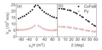
FIG. 3. (a) Group velocities of DE modes at room temperature as a function of applied field. Filled (open) circles denote CoFeB (permalloy). (b) Spin wave group velocity as a function of angle  $\beta$  when the in-plane field amounts to  $\mu_0 H = 20$  mT.
