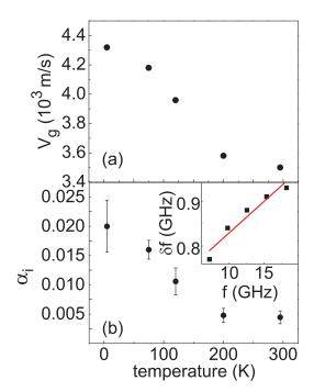
FIG. 5. (a) Group velocity measured on CoFeB in a perpendicular field of 1.9 T at different temperatures T. The eigenfrequency varies from 5.6 GHz to 7.2 GHz when T increases from 5 to 295 K. (b) Temperature dependence of intrinsic damping parameter  $\alpha_i$ . The inset shows  $\delta f$  vs f(H) at 295 K. The line reflects Eq. (2) leading to  $\alpha_i = 0.007$ .
