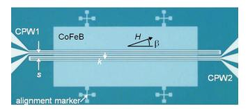
FIG. 1. Microscopy image of a CoFeB mesa with two integrated coplanar waveguides (CPWs). The center-to-center separation s of the two CPWs is 12  $\mu$ m. Orientations of in-plane magnetic field H and wave vector k are sketched.
