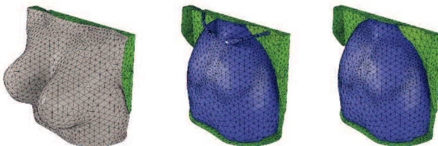
Figure 2: Meshing of the breast anatomy. Left: whole body model meshed with tetrahedrons, middle: fixed boundaries for the model with clavicles, right: fixed boundaries for the model without clavicles. The system boundaries are shown in green.
