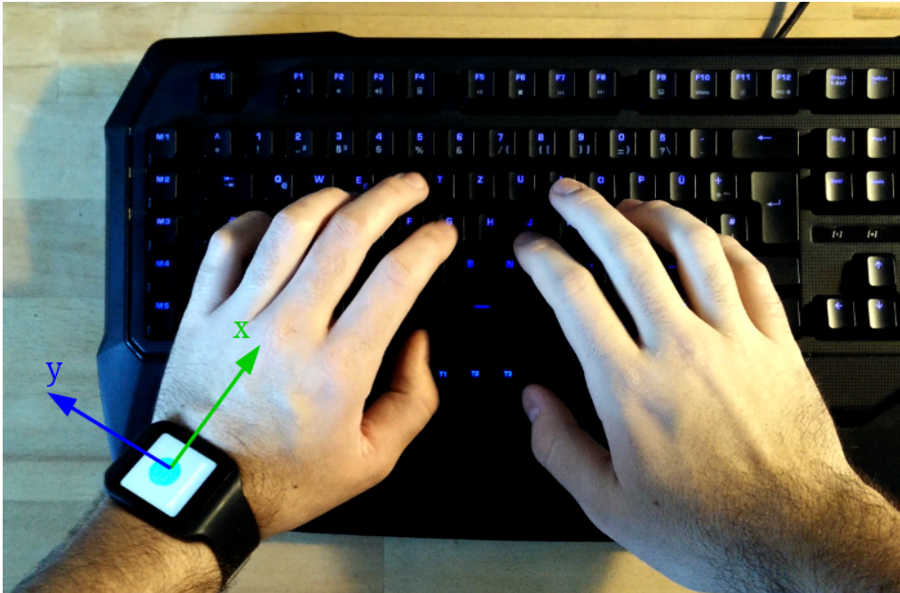
Figure 2.5: The coordinate system of a smartwatch while typing on a keyboard
