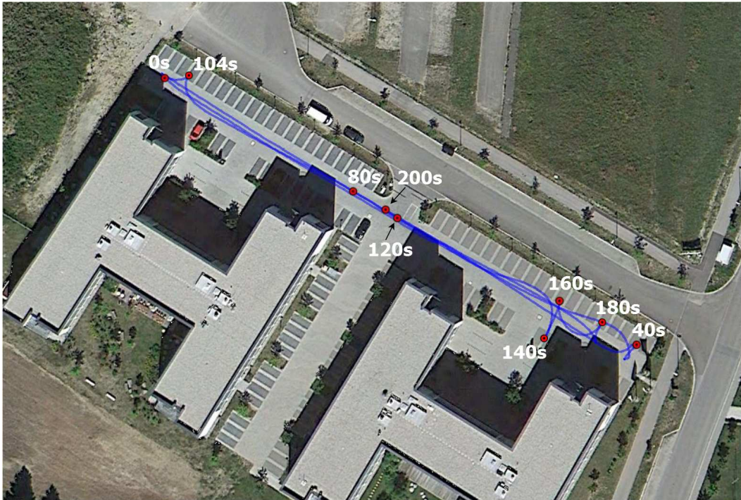
Figure 2.2: Track of car drive in front of the ESA/ AZO building in Oberpfaffenhofen. The track includes three reverse drives at 97 - 104 s, 140 - 160 s and 180 - 185 s.
