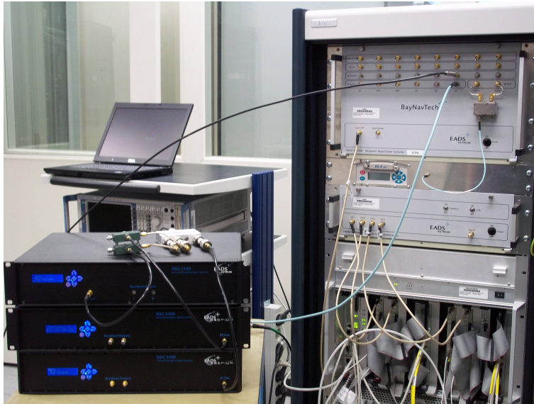
Figure 5.2: Photo of the experimentation. The BaySEF is on the right, the three NSGs are in the bottom left corner.
