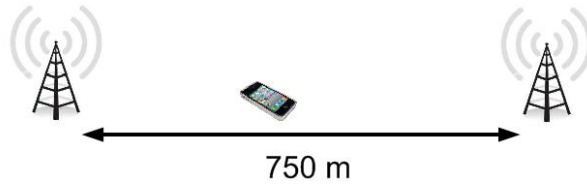
Figure 4.4: Two-base-station simulation scenario
