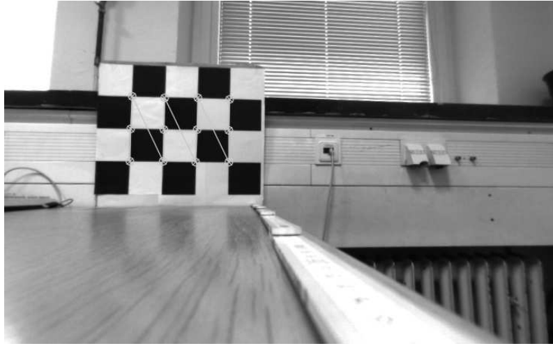
Figure 5.3: Corner Detection of a checkerboard for range estimation using a VI-Sensor
