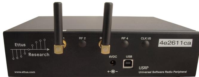
Figure 2.1: USRP1 device equipped with one daughterboard connected to two RF antennas and no external clock connected.
